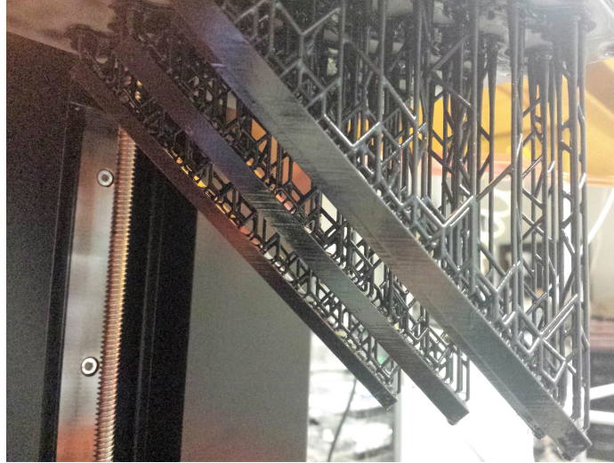
Figure 28: ES-SRR with support structures after printing
