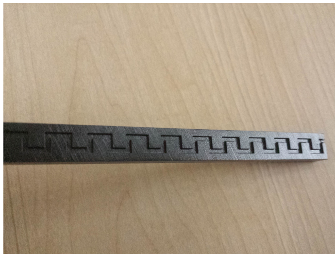
Figure 29: Cut-away view of ES-SRR to verify internal feature formation.
